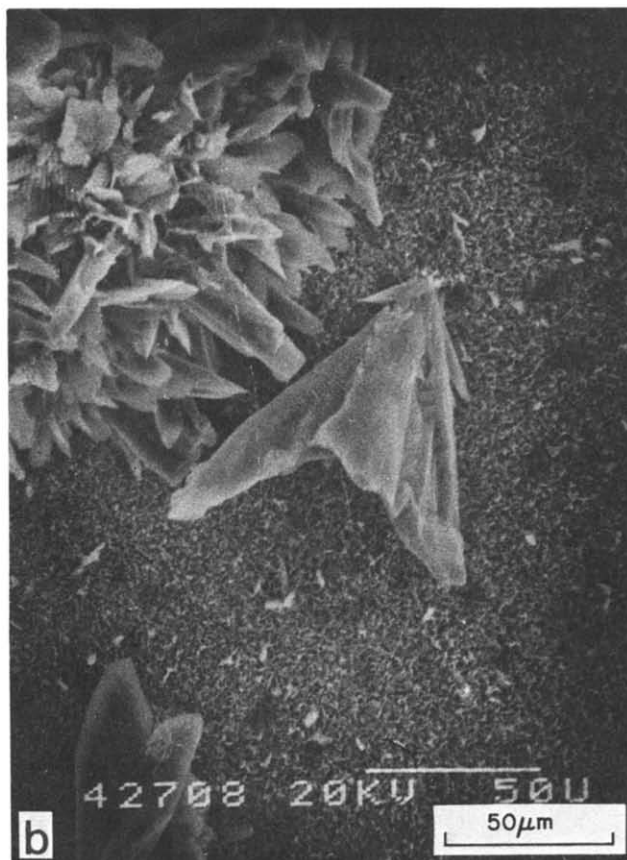
Figure 6 Scanning electron micrographs of orthorhombic polyoxymethylene, showing (a) scale-like and rod-like morphologies and (b) moth-shaped morphology
